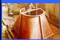
Using FastSHAPES®, this square to round transition was completed in less than 30 seconds ready to send to the burning machine. The development even included the line marking and number of degrees for forming every bend! Handles simple and complex shapes. All read directly into 2D and 3D CAD systems.
